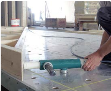
Small Pneumatic Pressor Even once disconnected the pneumatic ram upholds its 330 kg pressure
