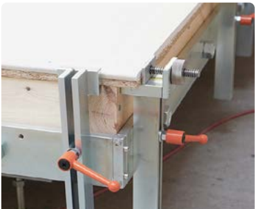
Panel Edge Stop Set the panel overlap directly on the stop
